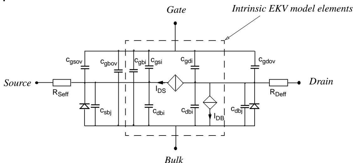
This figure represents the intrinsic and extrinsic elements of the MOS transistor. For quasistatic dynamic operation, only the intrinsic capacitances from the simpler capacitances model are shown here. However a charge-based trans-capacitances model is also available for computer simulation.
