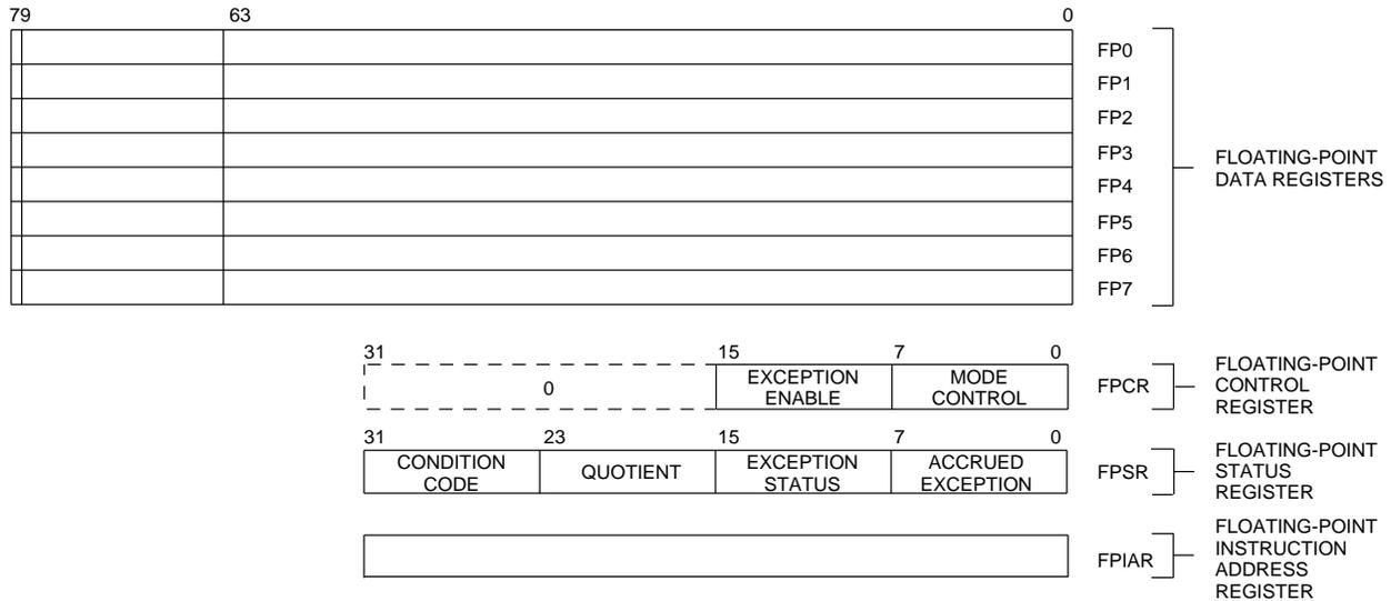
**Figure 1-2. M68000 Family Floating-Point Unit User Programming Model**
