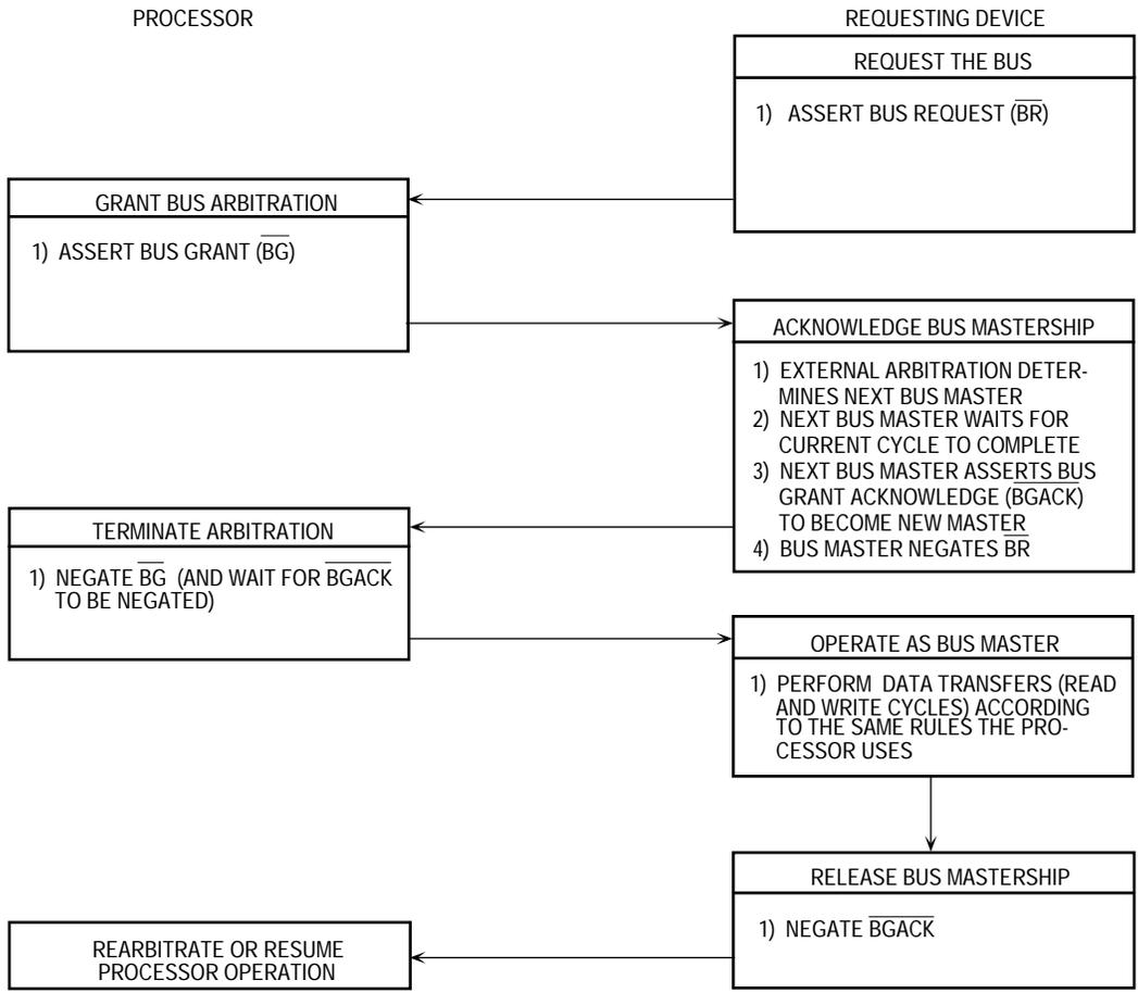
**Figure 5-13. 3-Wire Bus Arbitration Cycle Flowchart
