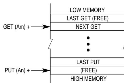
To implement the queue as a circular buffer, the relevant address register should be checked and adjusted. If necessary, do this before performing the put or get operation. Subtracting the buffer length (in bytes) from the register adjusts the address register. To implement growth of the queue from high memory to low memory, use the put address register indirect to put data into the queue and get address register indirect to get data from the queue.
