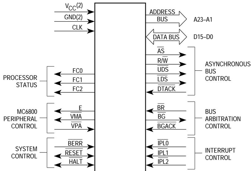
**Figure 3-1. Input and Output Signals
