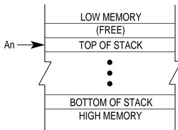
To implement stack growth from low memory to high memory, use  $(An) +$  to push data on the stack and  $-(An)$  to pull data from the stack. After either a push or pull operation, the address register points to the next available space on the stack. .
