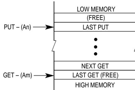
To implement the queue as a circular buffer, the get or put operation should be performed first. Then the relevant address register should be checked and adjusted, if necessary. Adding the buffer length (in bytes) to the address register contents adjusts the address register.
