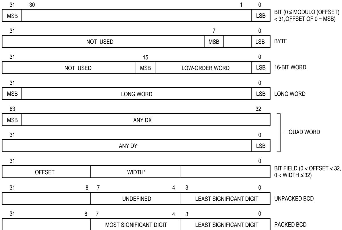
\* IF WIDTH + OFFSET > 32, BIT FIELD WRAPS AROUND WITHIN THE REGISTER.
