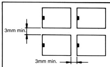
**Note:** Proper spacing is necessary to dissipate heat build-up from individual relays. Other than this, there are normally no restrictions depending on application. Please contact Omron for details.
