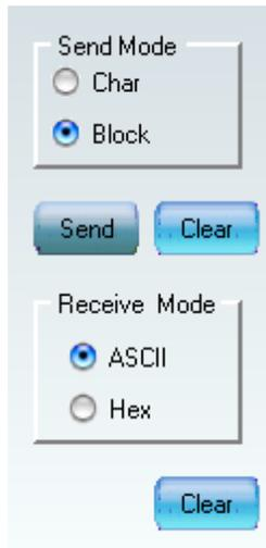
The serial controls are located at the bottom right of the GUI. The Send Mode block affects communication in the Send Console, while the Receive Mode block affects the Receive Console display.
