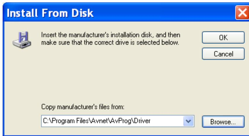
Figure 13 – Hardware Wizard Install From Disk Dialog
