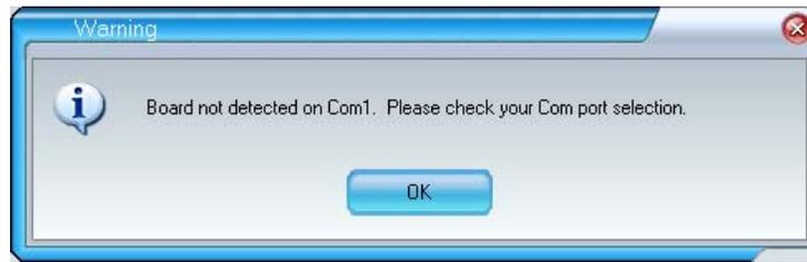
**Figure 19 – Board not connected Warning Dialog**
