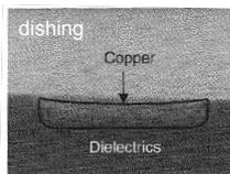
$w = 2 \mu\text{m}, t = 0.5 \mu\text{m}$  Cu line
