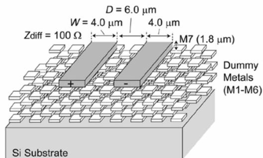
Open question: How do dummy metal fills affect transmission lines and passives ?
