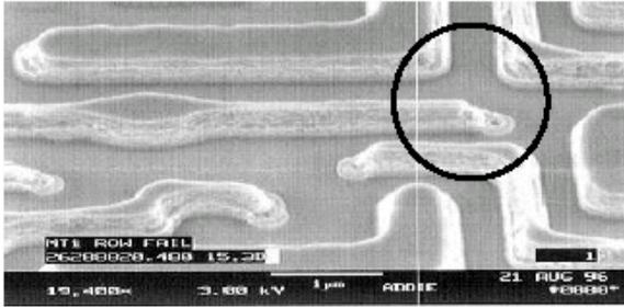
This top down SEM image was taken without any OPC. The pullback over the contact is clearly seen
