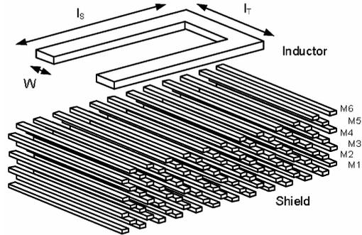
Borjesson et al., "VCO design for 60 GHz applications using differential shielded inductors in 0.13 μm CMOS," IPRC'08
