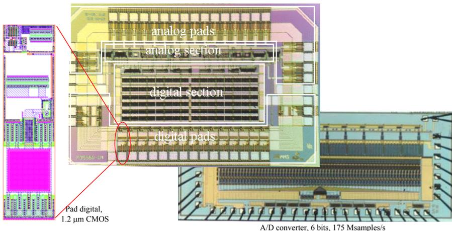
A/D converter, 6 bits, 175 Msamples/s
