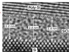
Oxide variations over a 20 Å nominal oxide thickness
