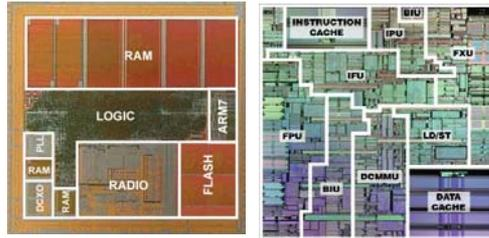
Floorplan of a communications SoC (left) and microprocessor (right)
